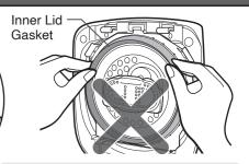
Do not forcibly pull the Inner Lid Knobs or Inner Lid Gasket toward you without pressing the Inner Lid Set Holder. May cause the Inner Lid Set and Outer Lid to break.
